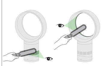
Look for blockages in the air inlet holes. Use a soft brush to remove debris.
